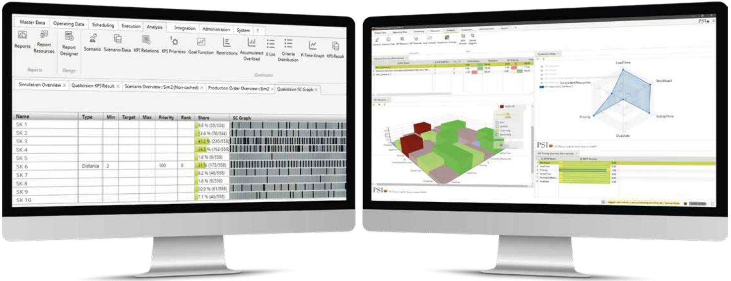
Figure 2: Qualicision AI Framework—Sequencing with order property distribution and scheduling with 3D KPI relationship matrix, KPI viewer, KPI preference settings.
